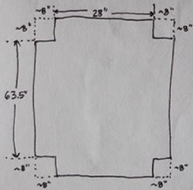
② Sew edges of each square cutout (right sides together, 1/4" seam allowance) together to make a box shape.
